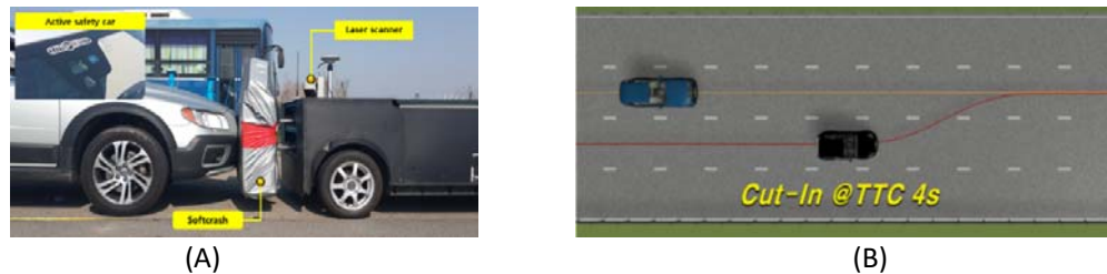
Fig. 2. (A) Active safety car test environment, (B) Cut-in scenario for the test.
