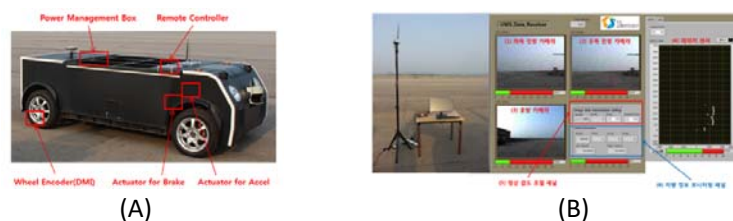
Fig. 1. (A) Layout of target vehicle, (B) Control server and program.
