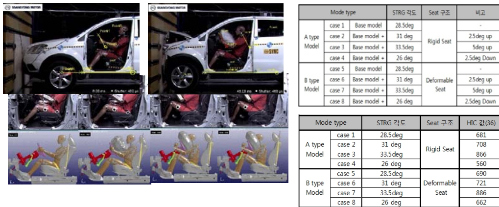
Fig. 1. Vehicle collision test tracking, CAE model setting table and Head injury results.
