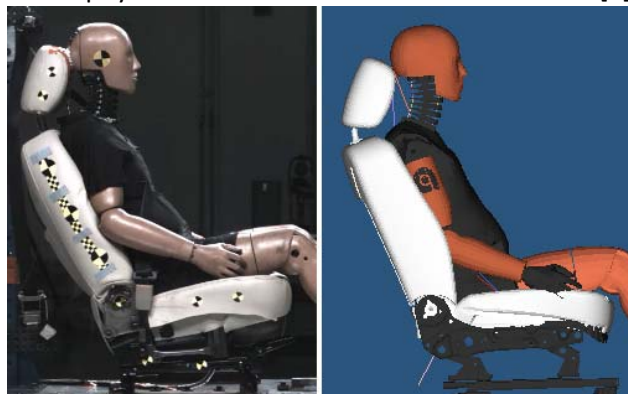
Fig.1. Whiplash sled test at 60ms (left) and the sled test simulation at 60ms (right)
