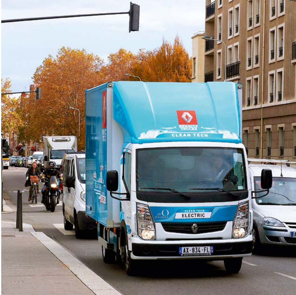
Quiet in the city. Renault Maxity Electric can run for 100 km on a single charge.
