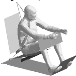
Fig. 3. HUMOS2LAB baseline model in the impactor test configuration (Load case A1).
