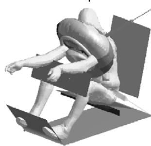
Fig. 3. HUMOS2LAB baseline model in the impactor test configuration (Load case A1).
