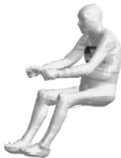
Fig. 3. HUMOS2LAB baseline model in the impactor test configuration (Load case A1).
