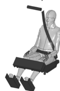
Fig. 7. THUMS baseline model in frontal sled test with belt (Load case D1).
