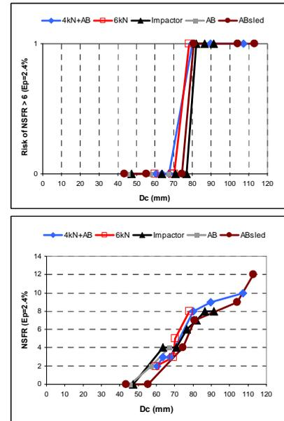
Fig. 4b. Risk curves (top) and injury curves (bottom) of Number of Fractured Ribs > 6 with Dc as injury criterion. Results obtained with HUMOSLAB2 model assuming a plastic strain failure threshold of 2.4%, representing a stronger subject.
