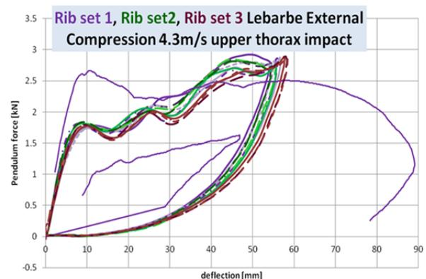
Fig. 7b. Test results compared to Lebarbe corridors
