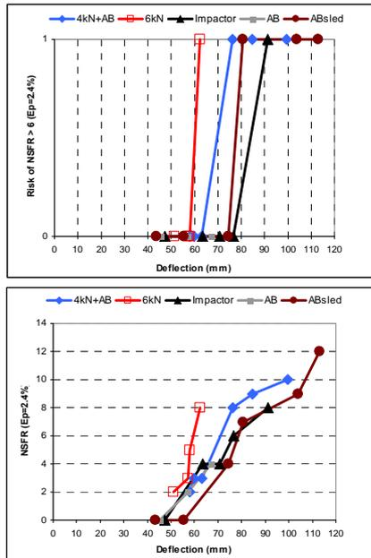
Fig. 4a. Risk curves (top) and injury curves (bottom) of Number of Fractured Ribs > 6 with sternal deflection as injury criterion. Results obtained with HUMOSLAB2 model assuming a plastic strain failure threshold of 2.4% representing a stronger subject.
