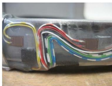
Fig. 9b. Detail of gage implementation
