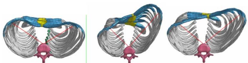
Fig. 3b. Examples of ribcage deformation shape under different loading types based on the HUMOS2LAB simulations. From left to right: airbag only, 6kN load limiter only, 4kN load limiter + airbag,
