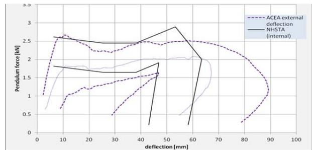
Fig. 6b. Comparison of NHTSA and Lebarbe corridors for 4.3m/s 23.4kg pendulum test
