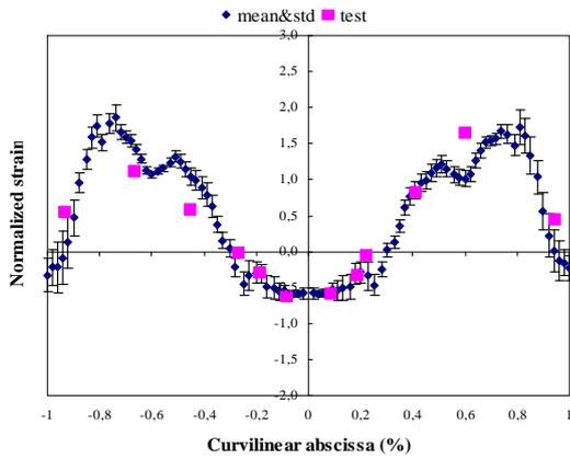
Fig. 2a Comparison of the strain profile for the 5th rib between the HUMOS2LAB model and the cadaver tests under static airbag loading performed by Trosseille et al. 2009 [47].
