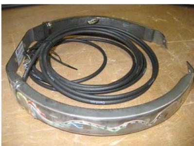
Fig. 9a. Example of rib with gages
