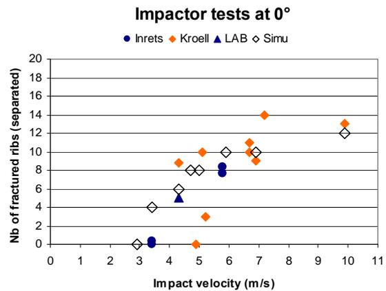
Fig. 2b. Number of fractured ribs versus loading severity for impactor tests: comparison between the HUMOS2LAB model and the experimental data (Kroell et al. 1974 [49], Bouquet et al. 1998 [47], Trosseille et al. 2009 [48]).
