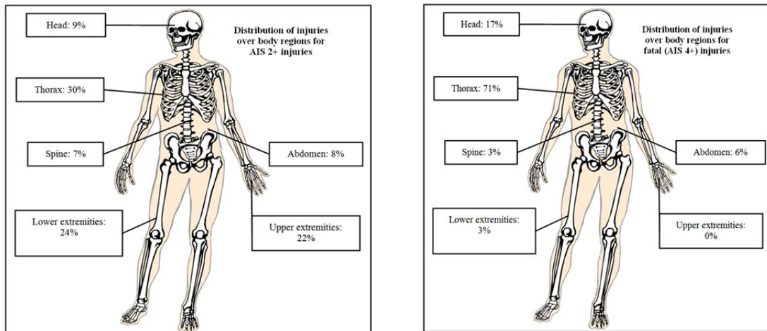
Fig. 1. (a) Distribution of AIS  $\geq 2$  and (b) AIS  $\geq 4$  injuries over body regions to car occupants sitting in front seats in frontal impacts for cars manufactured between 1996 and 2004 [3].
