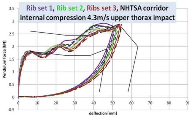
Fig. 7a. Test results compared to NHTSA corridors
