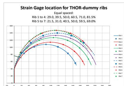
Fig. 9c. Gage positions (only left half)
