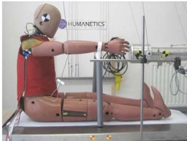
Fig. 6a. Set-up frontal impactor test
