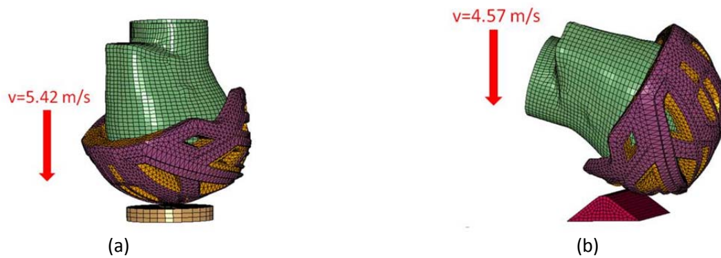
Fig. 7. Illustration of the simulation of standard impact tests against two anvils: (a) Flat anvil, (b) Kerbstone anvil
