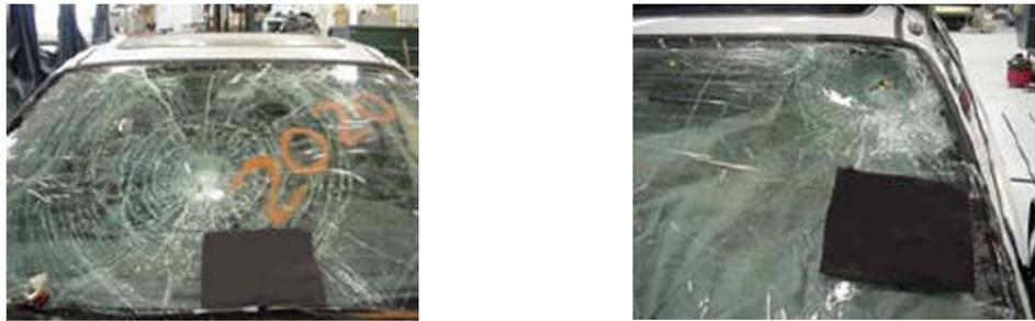
Figure 3 Fracture pattern of windshield during headform impact tests
