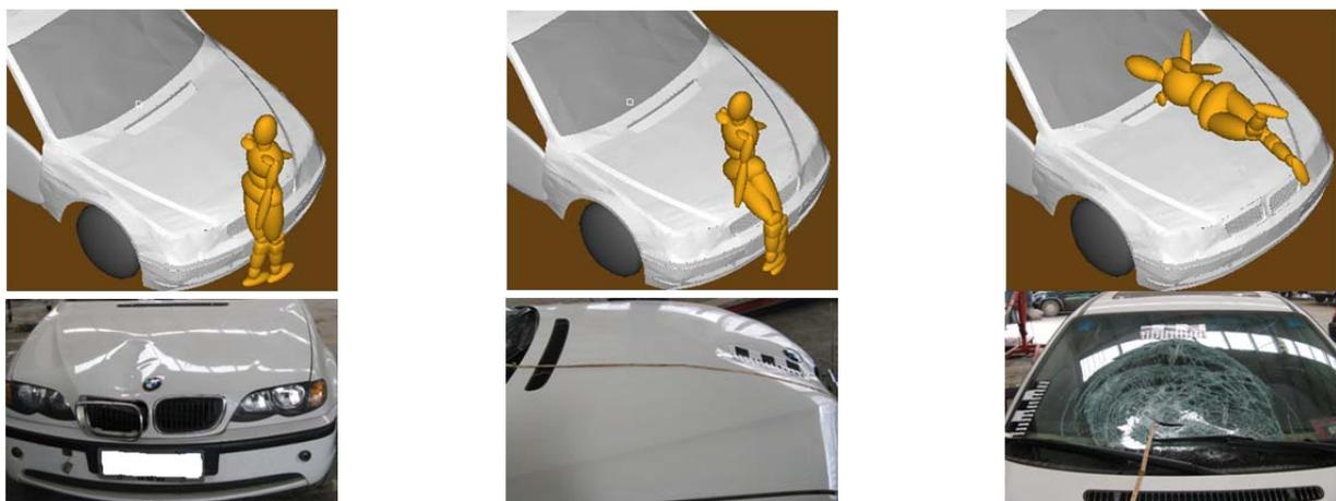
Figure 10 Illustration of the simulated pedestrian kinematics and comparison to real world observation for case IVAC 14
