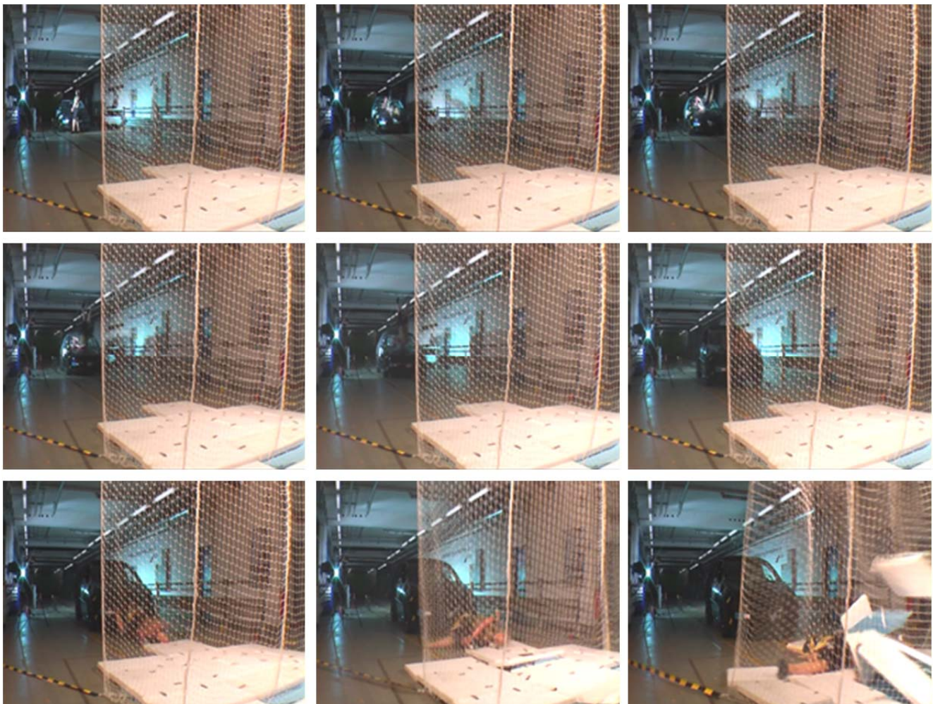
Fig. 27. Polar-II dummy test with a collision speed of 40 km/h (UDV, German Insurers Accident Research)
