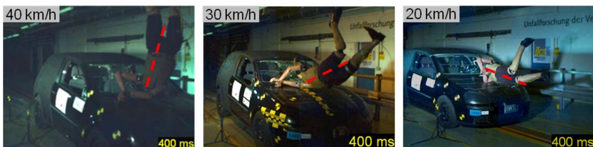
Fig. 26. Polar-II dummy tests with different collision speeds (50th percentile male)
