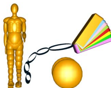
Fig. 6 - Variation of Windscreen Angle, shown in 5° steps, from 20° to 55°.
