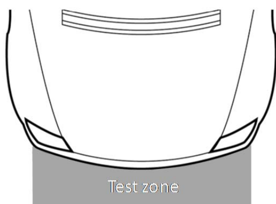
Fig. 10. Representative GTR 9 bumper test zone for case vehicle designs
