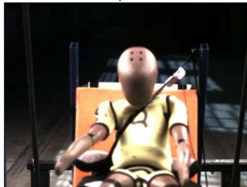
belt position observed in most of the cases after initial loading (belt moved upwards and is not aligned with deflection sensor)
