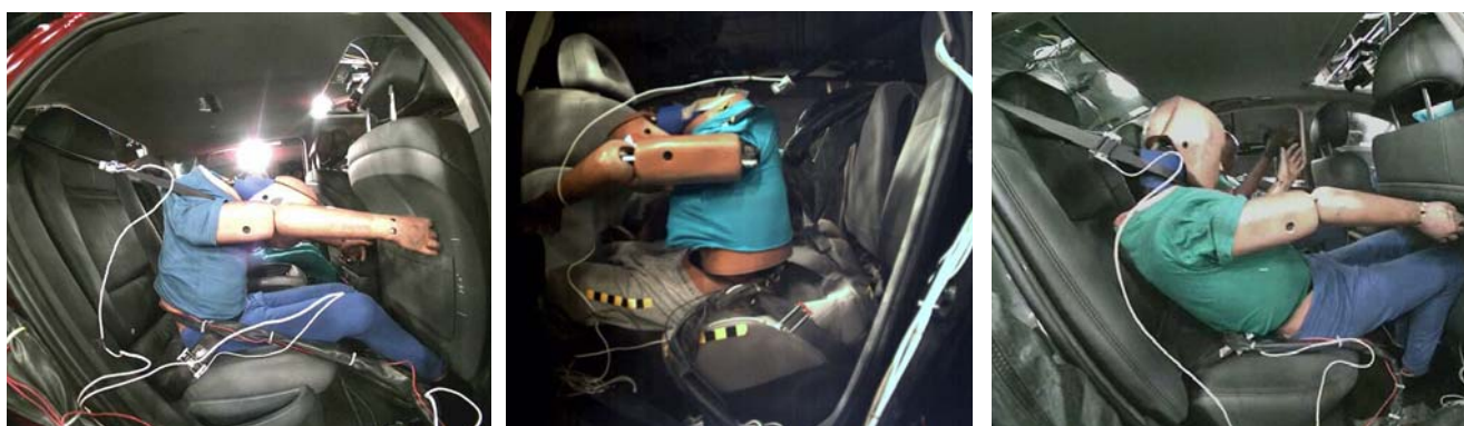
Fig. 6 Examples of typical kinematic responses observed in the rear seats of vehicles at peak excursion.
