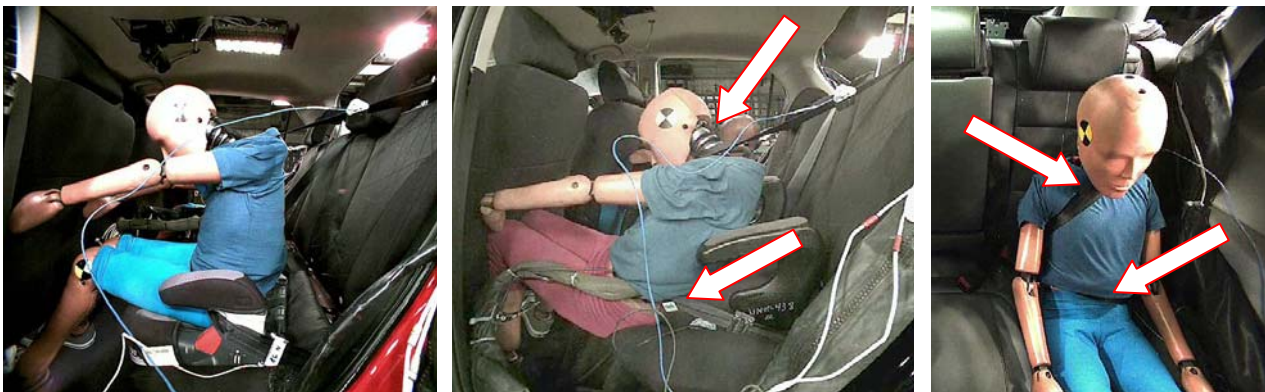
Fig. 11 Examples of “good” booster on the left; “poor” booster in the center and poor seat on the right.
