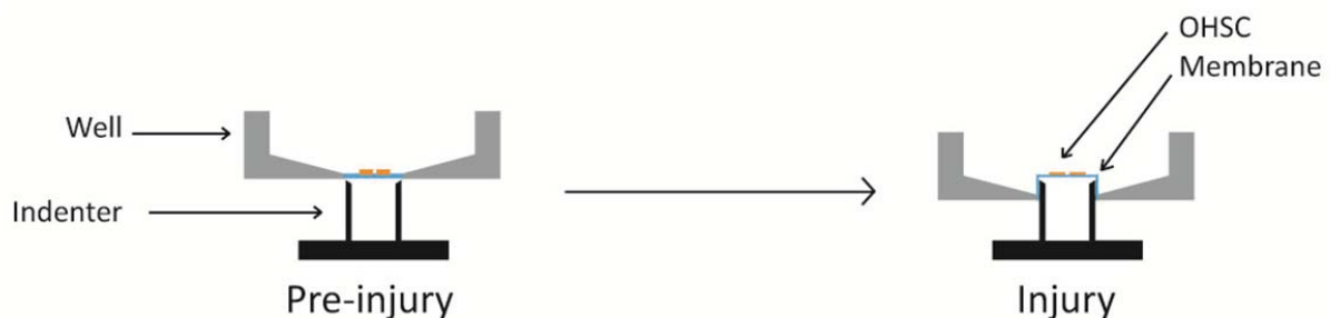
Fig. 1. Immediately prior to injury wells were clamped on the injury device and the membrane was lowered to the surface of the indenter. During injury, an equibiaxial strain was imparted to the OHSC by displacing the well and silicone tissue-substrate over a hollow, cylindrical indenter.
