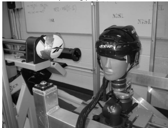
Fig. 1. Linear impactor system used to simulate the shoulder impact condition.
