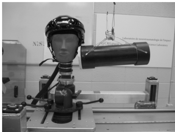
Fig. 3. Pendulum impact system used to simulate the punch impact condition.
