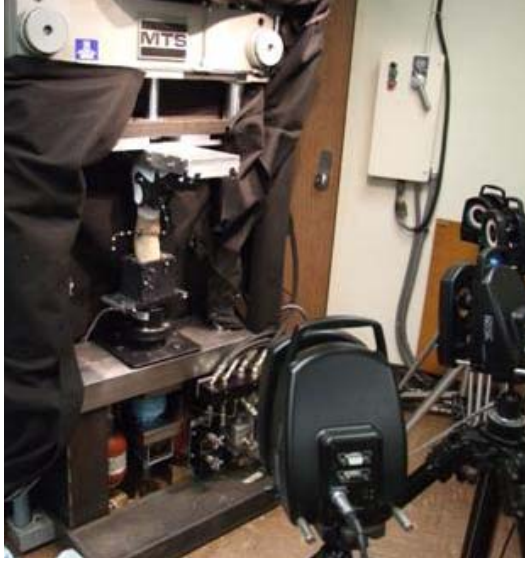
Fig. 3. Human cadaver ankle mounted in a servo-hydraulic testing machine. Vicon motion capture was used to track motion of the talus [28].
