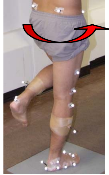
Fig. 4. Marker set of the Oxford Foot Model. The subjects performed a single-legged, external rotation of the foot, i.e. internal rotation of the body [30].
