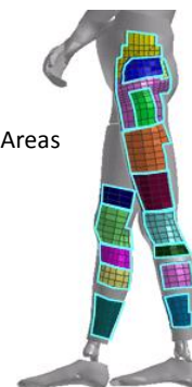
Fig. 9. Segmentation of Small Region in Baseline PFT Model for Vehicle C
