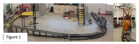
to cause a realistic tip-over. A Hybrid III dummy was modified and positioned in the cabin to approach the human dynamics in the precise conditions of side ejection. The modified dummy was validated by comparing its dynamic behaviour to human subject responses during tests
