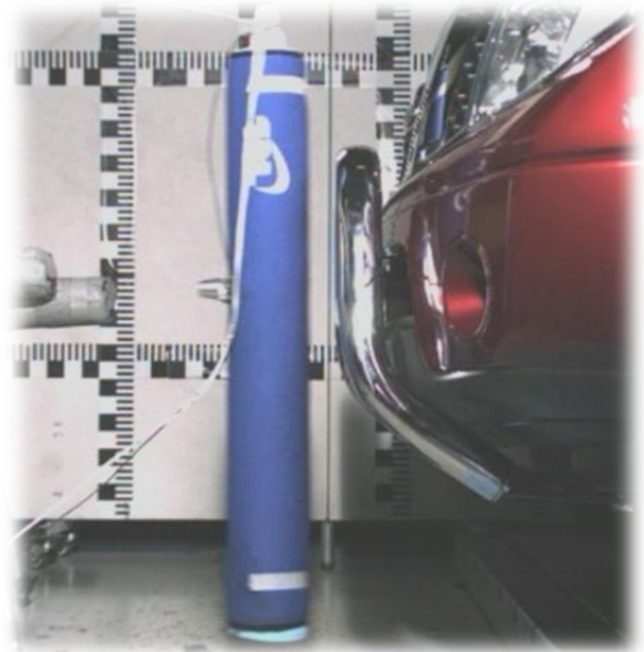
Fig. 6. Physical object - Nissan Navara and legform impactor during validation test
