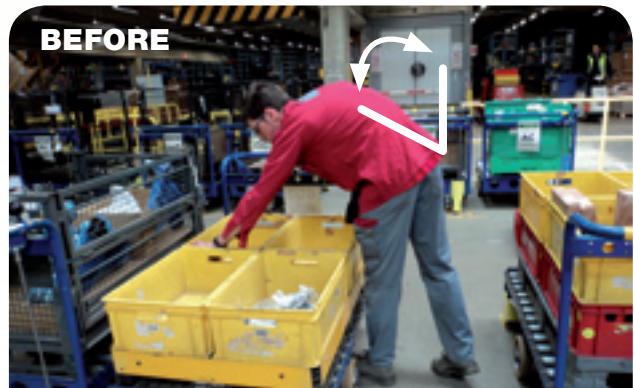
Before: The team member frequently bends forward to reach parts from the container.
